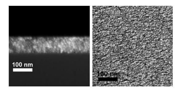
Electron microscopy (cross-section, left, and facing view) shows an even distribution of indium titanium oxide nanocrystals essential for a highly conductive, transparent thin film. Credit: Sun Lab/Brown University
