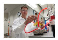
In the Materials Engineering Research Facility's process research and development lab, Argonne chemist Trevor Dzwiniel sets up a reaction calorimeter, which precisely measures how much heat a chemical reaction generates. This vital information is used to assess the scalability and safety of a reaction or process.
