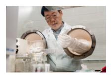
Argonne material engineer YoungHo Shin prepares a coin cell battery in a glovebox in the Materials Engineering Research Facility. Once it is prepared, the battery can be tested to determine the energy output characteristics of a cathode material for lithium-ion batteries.
