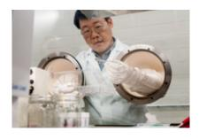
Argonne material engineer YoungHo Shin prepares a coin cell battery in a glovebox in the Materials Engineering Research Facility. Once it is prepared, the battery can be tested to determine the energy output characteristics of a cathode material for lithium-ion batteries.
