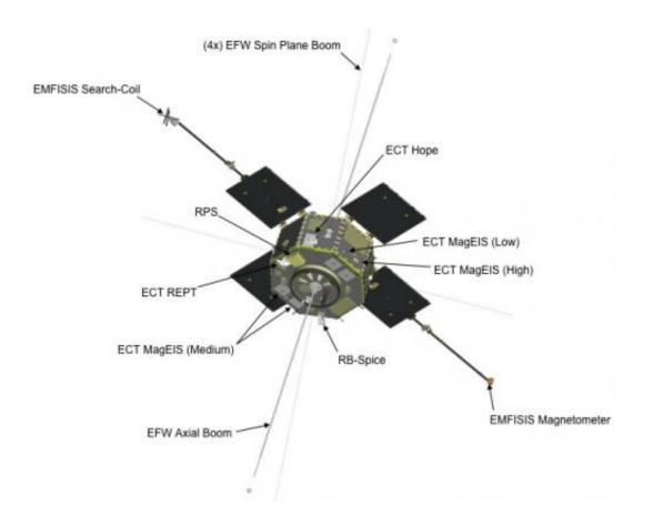
Each of the two Storm Probes is bristling with sensors to count energetic particles, measure plasma waves, and detect electromagnetic radiation.
