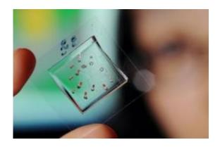
Georgia Tech associate professor Hang Lu holds a microfluidic chip that is part of a system that uses artificial intelligence and cutting-edge image processing to automatically examine large number of nematodes used for genetic research. Credit: Georgia Tech Photo: Gary Meek
