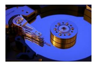
The interface between a slow non-volatile memory, like the hard drive in this picture, and fast electronic memory is a key bottleneck to computer performance.
