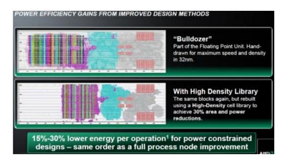
Steamroller is said to have been worked up as an overall enhancement to efficiencies in processing and power. Tom Verry, in *ExtremeTech*, writes in detail about what Steamroller is to bring:
