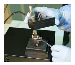
A researcher loads a sample into Lawrence Livermore National Laboratory's new fast polymerase chain reaction (PCR) instrument.
