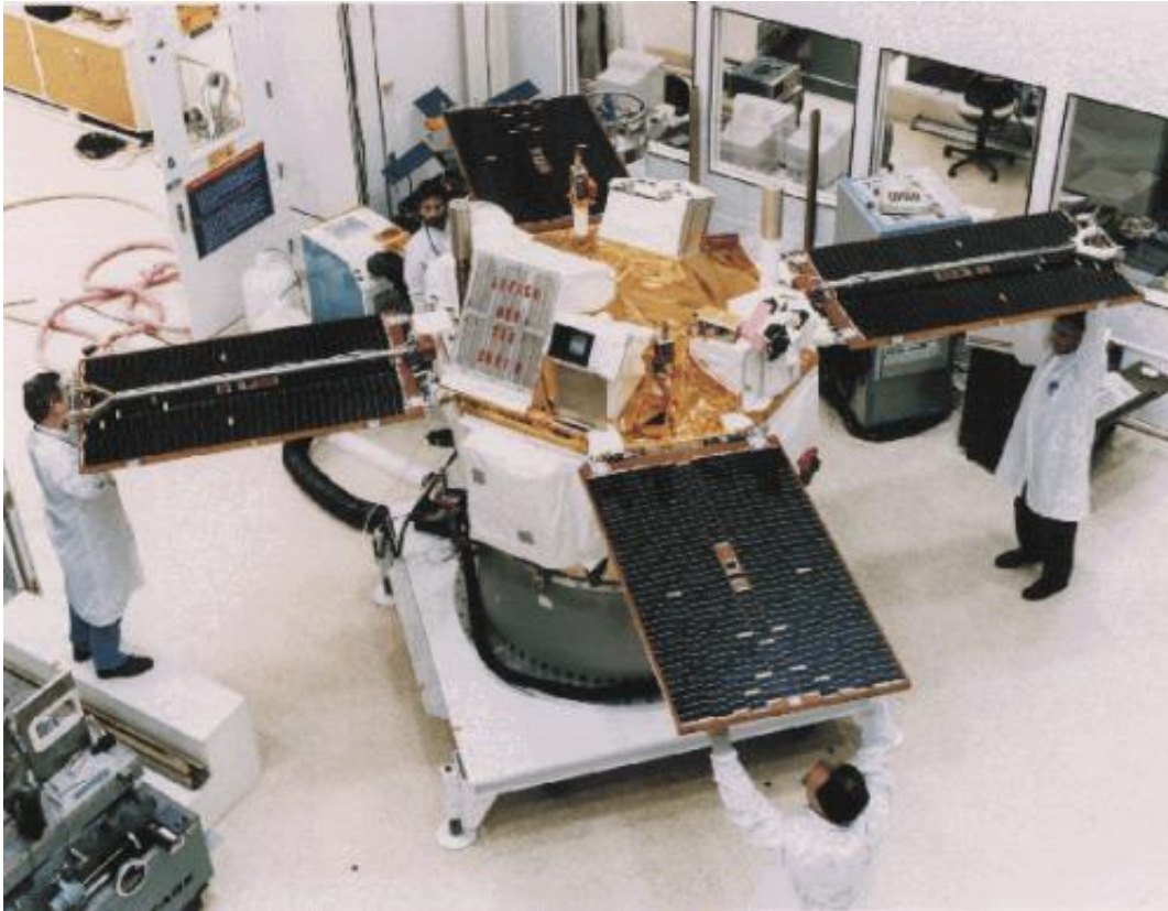
ACE under construction with scientists holding the solar arrays. Credit: Caltech
