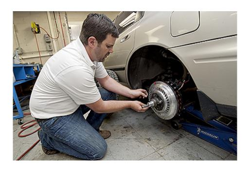
Jay Perry views the rotor he has removed from the stator, which is attached to the axle bearings. In the entire process, nothing alters the car'€™s bearings, brakes or suspension.
