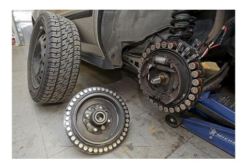
The plug-in hybrid retrofit kit is applied to a vehicle'€™s rear wheels. After switching on the traction motors, gas mileage can increase 50 to 100 percent.
