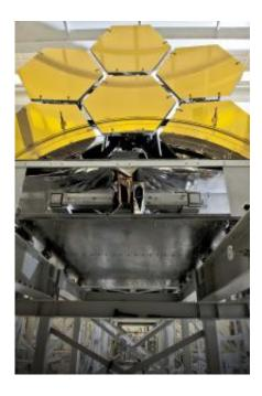
The gold layer coating, only a few millionths of an inch thick, enables the mirrors to best reflect the infrared light the telescope seeks. Credit: NASA's Goddard Space Flight Center/Chris Gunn
