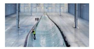
The B75 blade is the world's largest fiberglass component cast in one piece. The manufacturing process posed several challenges for the project team. In particular, the mold had to consist of two parts so that it could be transported.
