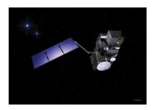
Sentinel-3 is being developed by ESA for the European Global Monitoring for Environment and Security programme. The mission's main objective is to measure sea-surface topography using radar altimetry, sea- and land-surface temperature using an advanced visible/thermal radiometer and ocean- and land-surface colour using a visible spectrometer. Credits: ESA-J. Huart
