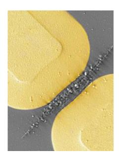
Image showing a scanning electron microscope image of damaged vanadium dioxide in the gap of a terahertz metamaterial made of gold. The damage results when strong field enhancement of incident terahertz radiation in the gaps leads to a rapid increase in the energy density following the field-driven insulator-to-metal transition. Image Credit: Mengkun Liu / Mario D'Amato
