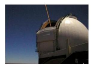
A laser beam aims skyward from the Keck II 10-meter telescope atop Mauna Kea in Hawaii, creating a sort of artificial "star" that, when coupled with an adaptive optics system featuring an adjustable mirror, can compensate for distortions in Earth's atmosphere and produce clearer space images. The laser guide star, used to measure the atmospheric distortions, excites sodium ions about 56 miles high. Photo courtesy Adam Contos (Ball Aerospace)
