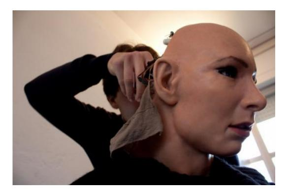
The robot's servo motors actuate the "face" in a different way, however. In contrast to human muscles, the robot servos are only capable of producing linear contractions. Human orbicular muscles, like the Orbicularis oculi and the Orbicularis oris, produce circular contractions. "The movement of this kind of muscles is reproduced using more than one servo motor in the most realistic way as possible."
