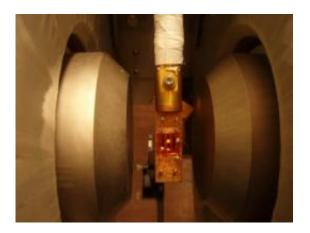
A new "spintronic" organic light-emitting diode glows orangish (center) when the device, chilled well below freezing, is exposed to a magnetic field from the two poles of an electromagnet located on either side of the device. University of Utah physicists report inventing the new kind of LED in the July 13 issue of the journal *Science*. Credit: Tho Nguyen, University of Utah
