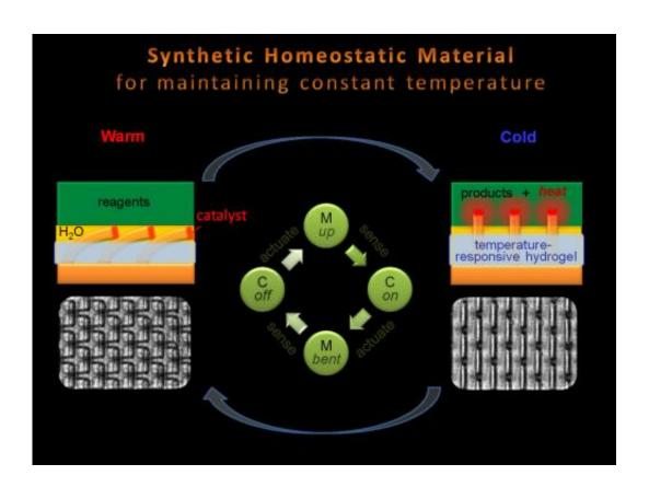
This is a schematic of the temperature-regulating SMARTS displaying a C-M feedback loop, in which mechanical action of T-responsive gel is coupled with an exothermic reaction. The sideview schematic and top-view microscope images depict "on-off" states of the reaction in the top layer. Credit: Laboratory of Joanna Aizenberg, Harvard School of Engineering and Applied Sciences
