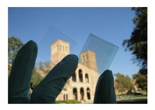
Transparent Solar Cells. Visibly Transparent Polymer Solar Cells Produced by Solution Processing
