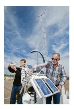
Tim Leonard, right, owner of Precision Solar Technologies Corp., and the company's project engineer, Tony Louderbough, do final adjustments on the instrumentation of a trailer-mounted solar weather station, called the Prospector Mule, at Sandia Labs. Precision Solar uses a tracking technology developed at Sandia. (Photo by Randy Montoya)
