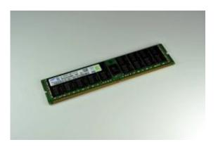
Samsung Electronics today announced that it has begun sampling the industry's first 16-gigabyte (GB) double data rate-4 (DDR4), registered dual inline memory modules (RDIMMs), designed for use in enterprise server systems.
