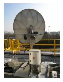
The SMART solution eliminates the need for complex antenna closed-loop controller/beacon receiver equipment. Combined with the use of off-the-shelf DC actuators and high-performance motor control electronics , the SMART project has demonstrated that the YELLOWSAT open-loop tracking solution is effective and reliable. Credits: ESA photo
