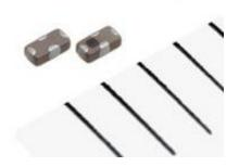
TDK Corporation has developed a multilayer band pass filter in size 1005 that is significantly smaller than the existing 1608 types.
