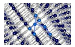
Hydrogen vacancy clustering in aluminum hydride (AlH3): The dark blue atoms represent the Al atoms in the regular AlH3 lattice, and the light blue atoms represent the Al atoms in the Al-rich region created by the clustering of hydrogen vacancies as hydrogen leaves the material. Credit: Van de Walle Group
