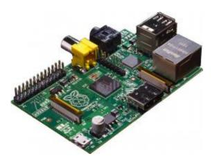
The Raspberry Pi is a credit-card sized computer that plugs into your TV and a keyboard. It's a capable little PC which can be used for many of the things that your desktop PC does, like spreadsheets, word-processing and games. It also plays high-definition video.
