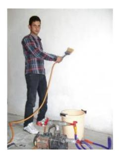
In this undated photo provided by the National Innovation Foundation, Jahangir Ahmad demonstrates his invention called Electric Painting Brush in India. The device pumps paint from a hose directly to the brush and never needs to be dipped into a can. (AP Photo/National Innovation Foundation)
