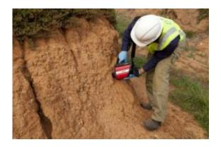
The RemScan device uses an infrared signal to directly measure petroleum contamination in soil.
