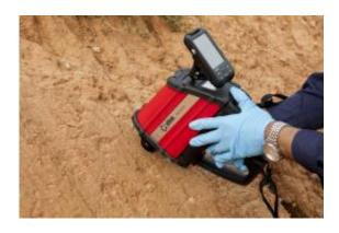
The RemScan device can measure petroleum contamination in soil with a simple pull of the trigger.
