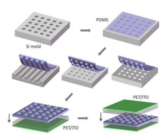
This schematic shows the fabrication process for patterned surfaces in the triboelectric nanogenerators and pressure sensors. A patterned silicon wafer serves as the mold for fabrication of PDMS thin films with micro-patterned features. Credit: Image courtesy of Zhong Lin Wang
