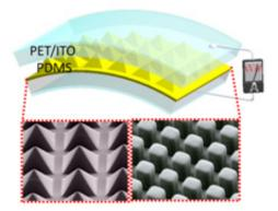
This diagram shows a new high-output, flexible and transparent trioboelectric nanogenerator produced from transparent polymer materials. Credit: Image courtesy of Zhong Lin Wang
