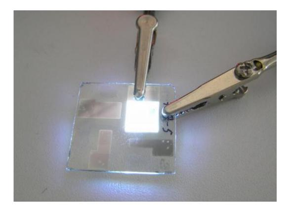
A white polymer light-emitting diode fabricated at the University of Groningen. Devices such as this suffer losses from charge traps in the materials. (Click image for high-resolution version. Credit: Herman Nicolai, University of Groningen
