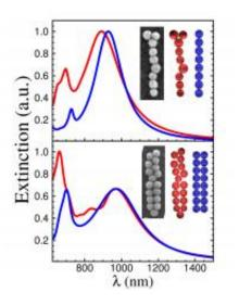
How far a wavelength of light can be transmitted along a gold nanoparticle chain to where it dies down (the "extinction" point) depends on the configuration of the repeat units - the nanoparticles themselves - according to Rice University researchers. Their study was intended to draw parallels between nanoparticle arrays and polymers that also depend on chemical repeat units for their characteristics. Credit: Liane Slaughter/Rice University
