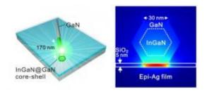
This is an illustration of the nanoscale semiconductor structure used for demonstrating the ultra-low-threshold nanolaser. A single nanorod is placed on a thin silver film (28 nm thick). The resonant electromagnetic field is concentrated at the 5-nm-thick silicon dioxide gap layer sandwiched by the semiconductor nanorod and the atomically smooth silver film. Copyright *Science*
