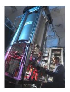
The caesium fountain clock, NPL-CsF2, which keeps the United Kingdom's atomic time, is located at the National Physical Laboratory in Teddington. The whole device is approximately 8.2 feet (2.5 m) high. Atoms are tossed up 3.2 feet (1 m) inside a microwave cavity, which is inside a vacuum vessel. The large external cylinder screens the atoms inside the clock from the relatively large and unstable external magnetic field. Credit: National Physical Laboratory; United Kingdom
