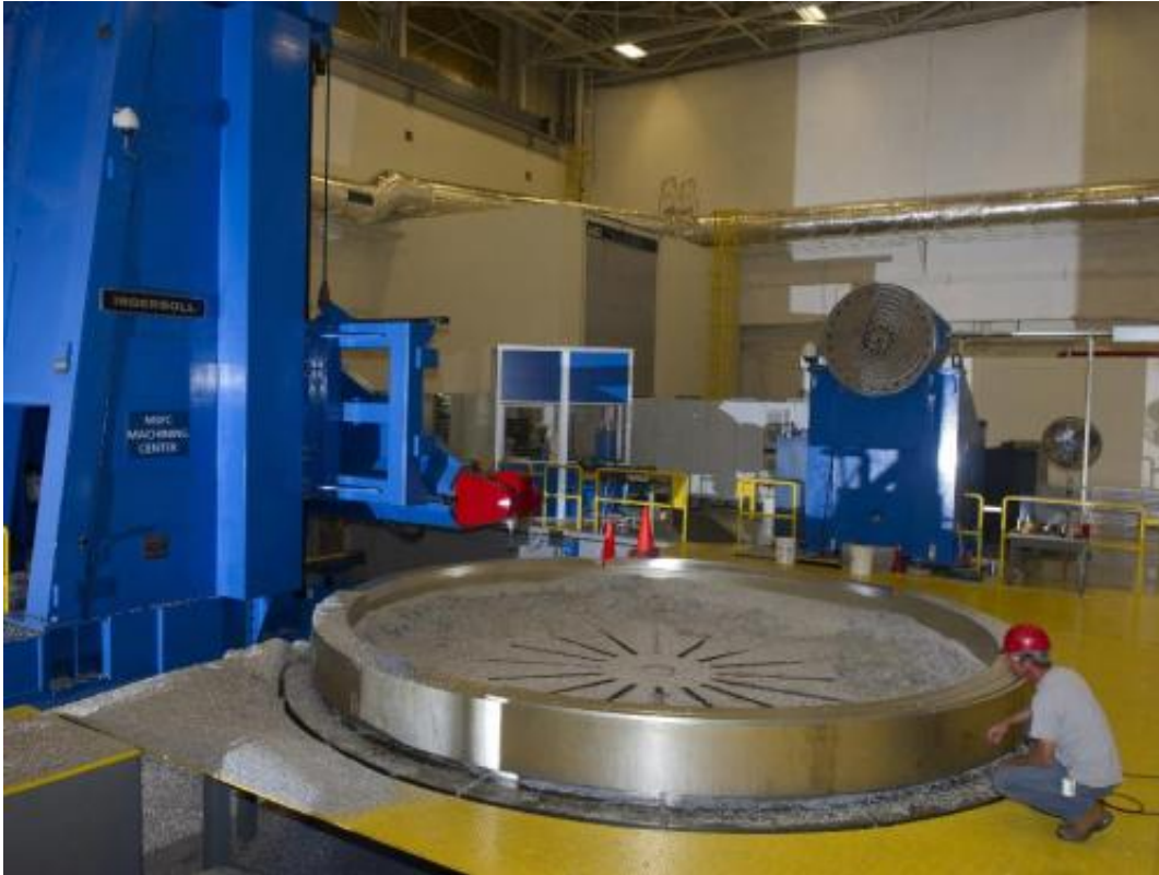
A Marshall Center machinist takes a close look at a recent cut on an aluminum adapter ring. Credit: NASA/MSFC
