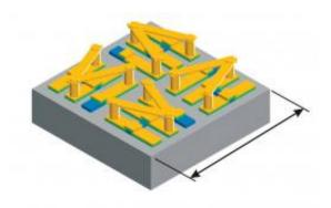
The schematic shows the chirality switching metamolecule consists of four chiral resonators with fourfold rotational symmetry. An external beam of light instantly reverses the metamolecule's chirality from right-handed to left-handed. Credit: Courtesy of Xiang Zhang, et. al
