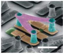
The top shows a scanning electron microscopy image of optically switchable chiral THz metamolecules. The bottom shows the purple, blue and tan colors represent the gold meta-atom structures at different layers, with the two silicon pads shown in green. Courtesy of Xiang Zhang, et. al
