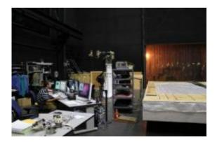
Precision honed to within +/-0.0018 inches tolerance across its surface, the Gravity Offset Table (shown right) will allow scientists to emulate the inertia of space in the laboratory using full-size spacecraft and robotic arms like the Front-End Robotic Enabling Near-Term Demonstration (FREND) arm pictured center. Credit: US Naval Research Laboratory
