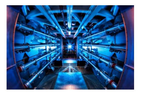
The preamplifiers of the National Ignition Facility are the first step in increasing the energy of laser beams as they make their way toward the target chamber. NIF recently achieved a 500 terawatt shot - 1,000 times more power than the United States uses at any instant in time.
