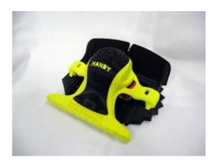
This functioning ice scraper was printed in 3-D using capabilities developed at the University of Dayton Research Institute.
