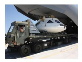
Image above: The Orion team loads a test version of the spacecraft into a C-17 in preparation for a parachute drop test at the U.S. Army Yuma Proving Ground in Arizona. The main objective of the latest drop test is to determine how the entire system would respond if one of the three main parachutes inflated too quickly. Credit: NASA
