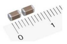
TDK Corporation has developed a multilayer ceramic chip capacitor that – in addition to its rated DC voltage of 630 V – can withstand a rated AC voltage of 500 VRMS for 60 s and 600 VRMS for 3 s. Thanks to its optimized internal electrode structure the new TDK C3216 and C3225 types exhibit superior AC withstanding voltage, allowing guaranteed ratings to be given not only for the customary DC voltages but also for AC voltages.
