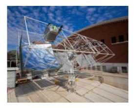
The "tracker" consists of a steel frame that ultimately will support eight mirrors, together generating enough electricity to power about four to five homes. The prototype has been modified since this picture was taken. Credit: Blake Coughenour
