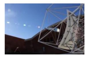
A dish-shaped mirror focuses sunlight onto a glass ball, which distributes it evenly onto an array of photovoltaic cells. Credit: Blake Coughenour
