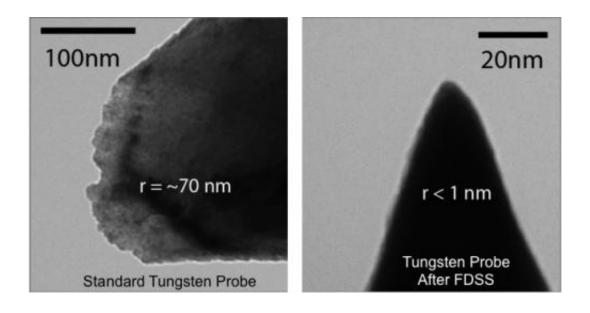
This is a traditionally etched tungsten STM probe (left), sharpened to a 1-nanometer point after bombarding it with ions (right). Credit: Joseph Lyding
