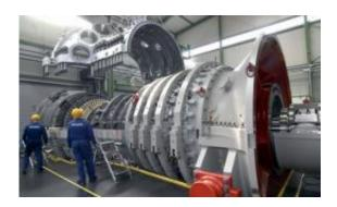
The SGT5-8000H gas turbine developed by Siemens forms the heart of the highly efficient combined cycle power plant with district heat extraction in Düsseldorf, Germany. With an electrical unit output of around 595 megawatts (MW) and a net .
