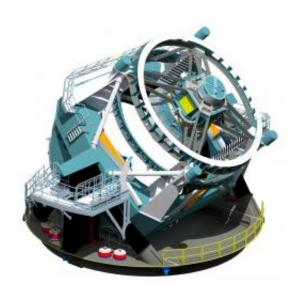
An artist's rendering of the proposed Large Synoptic Survey Telescope. The 8.4-meter LSST will use a special three-mirror design, creating an exceptionally wide field of view and will have the ability to survey the entire sky in only three nights. Credit: LSST Corporation
