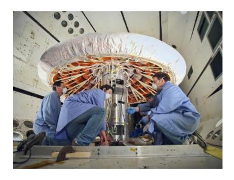
Engineers checked out the Inflatable Reentry Vehicle Experiment after the successful completion of an inflation system test. Credit: NASA/ Sean Smith
