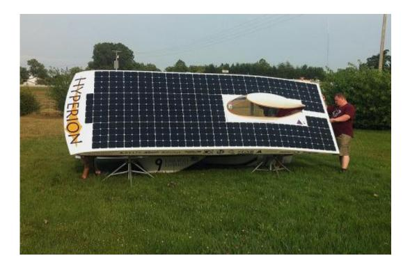
Hyperion's solar array is tilted to the sun for a better battery charge. Credit: Team PrISUm
