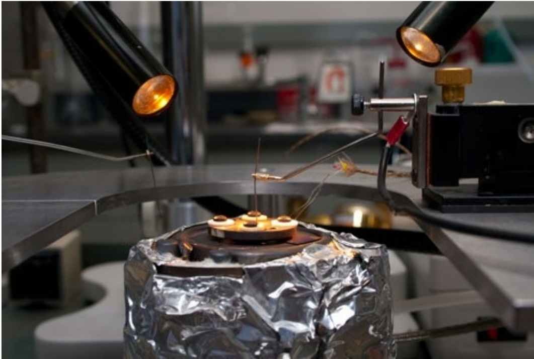
The laboratory setup for testing solid-oxide fuel cells. Image credit: Caroline Perry, SEAS Communications
