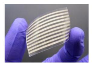
Researchers from North Carolina State University have developed highly conductive and elastic conductors made from silver nanowires. These elastic conductors can be used to develop stretchable electronic devices. Credit: Yong Zhu, North Carolina State University
