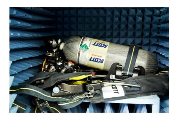
A PASS unit and air pack are placed in an anechoic chamber for testing.
