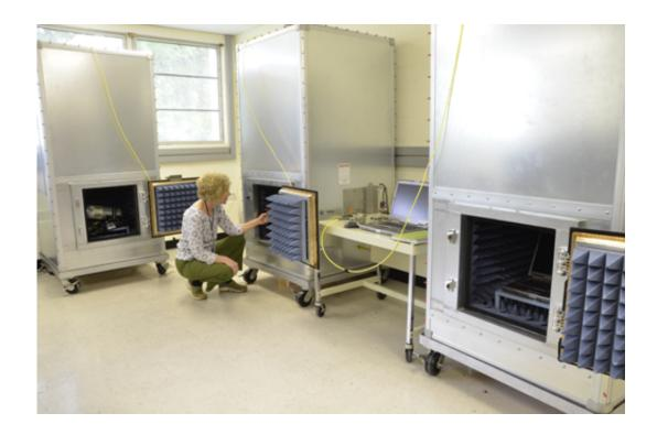
Researcher Kate Remley examines the middle chamber containing a repeater unit in a "one hop" communications test. The PASS is in the cabinet at left, and the base station is in the cabinet at right.
