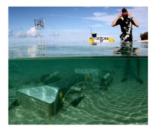
This photo shows one of the cpFOCE flumes underwater, with the wind-power generator and floating computer control system in the background. Credit: David Kline
