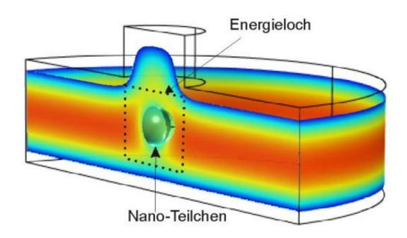
This is a cross-section through two chip-sized glass plates in which a nano particle is trapped in an energy hole (or "potential well" to use the scientific term). The colored fields show the different charges in the electrostatic field. The red zone signifies a very low charge, while the blue edges have a strong charge. Credit: University of Zurich
