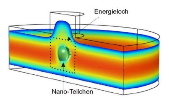
This is a cross-section through two chip-sized glass plates in which a nano particle is trapped in an energy hole (or "potential well" to use the scientific term). The colored fields show the different charges in the electrostatic field. The red zone signifies a very low charge, while the blue edges have a strong charge. Credit: University of Zurich
