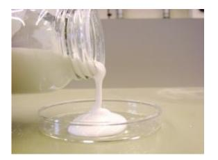
Heat can damage the batteries of electric vehicles – even just driving fast on the freeway in summer temperatures can overheat the battery. An innovative new coolant conducts heat away from the battery three times more effectively than water, keeping the battery temperature within an acceptable range even in extreme driving situations.
